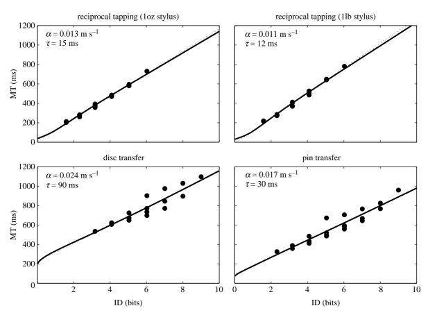
Figure 3. The speed-accuracy trade-off of the delayed circuit for parameters within the range estimated for each of Fitts' experiments. The solid line represents the speed-accuracy trade-off for the circuit. The broken line represents linear regression.
