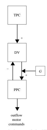
Figure 1. Network diagram of the VITE circuit with connections indicated as excitatory or inhibitory. TPC, target position command; PPC, present position command; DV, difference vector; G, gain signal.
