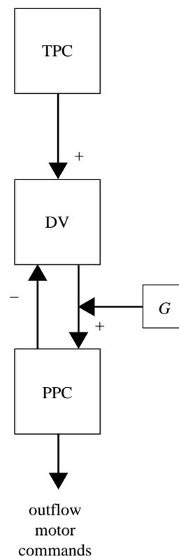
Figure 1. Network diagram of the VITE circuit with connections indicated as excitatory or inhibitory. TPC, target position command; PPC, present position command; DV, difference vector;  $G$ , gain signal.
